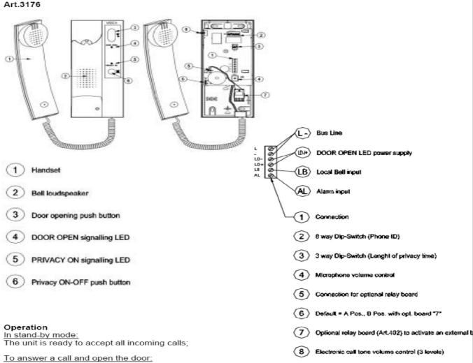
Pick the handset up and speak with the visitor (or concierge); press the "Key" button (if it is an external call) to open the door (an acoustic signal will be emitted and the door will be opened for the time programmed) or replace the handset to end the conversation; if the call is local (local bell), the call tone will have a different tonality from the main one
