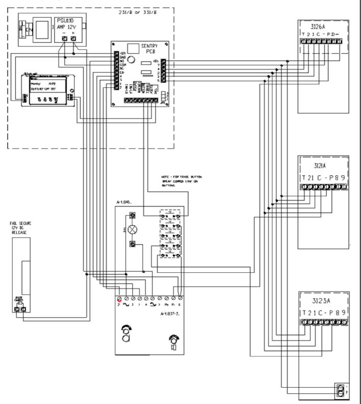
This diagram shows a single entrance vandal resistant door panel connected to multiple apartments. The lock release shown is fail safe and a break glass is connected in line. We recommend bringing all telephones back to one point (i.e. control cabinet) on this type of installation.
