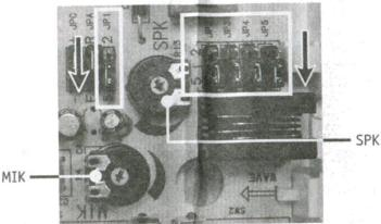
In case of traditional speech signal, set the trimmers MIK and SPK as shown in the photo. In case of electronic speech signal, rotate all the trimmer SPK clockwise.
